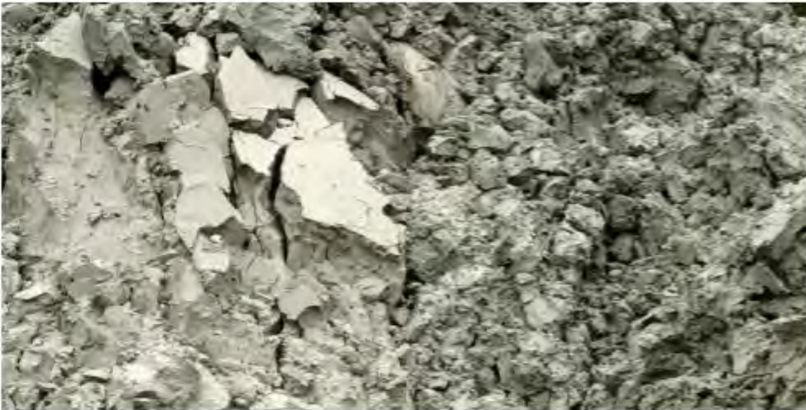
Figure 1 The left panel above is from a natural clay deposit, and it illustrates on a macroscopic scale that clays are anisotropic materials. The right panel is an electron microscope image of vermiculite clay demonstrating its lamellar structure on the nano-scale, reminiscent of graphene, which is one of the main characteristics of clay minerals.
